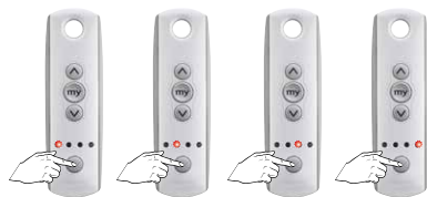
Telis 4 with blinds programmed to channel 1 up to 4
